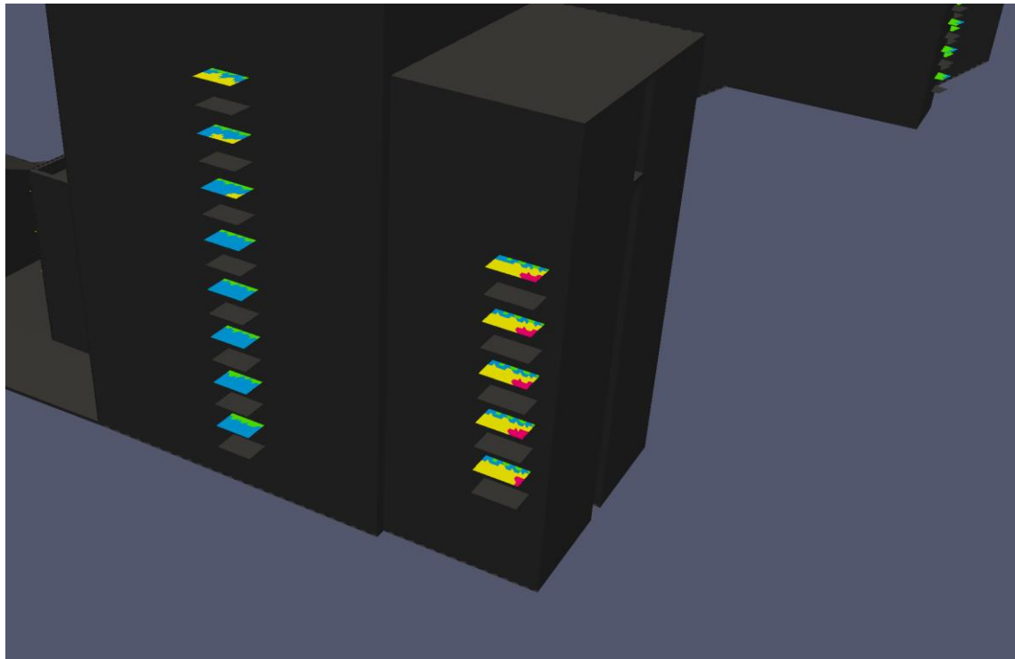
Figure 53 Image showing walking use wind conditions at south-east balconies on Building B during windiest season
