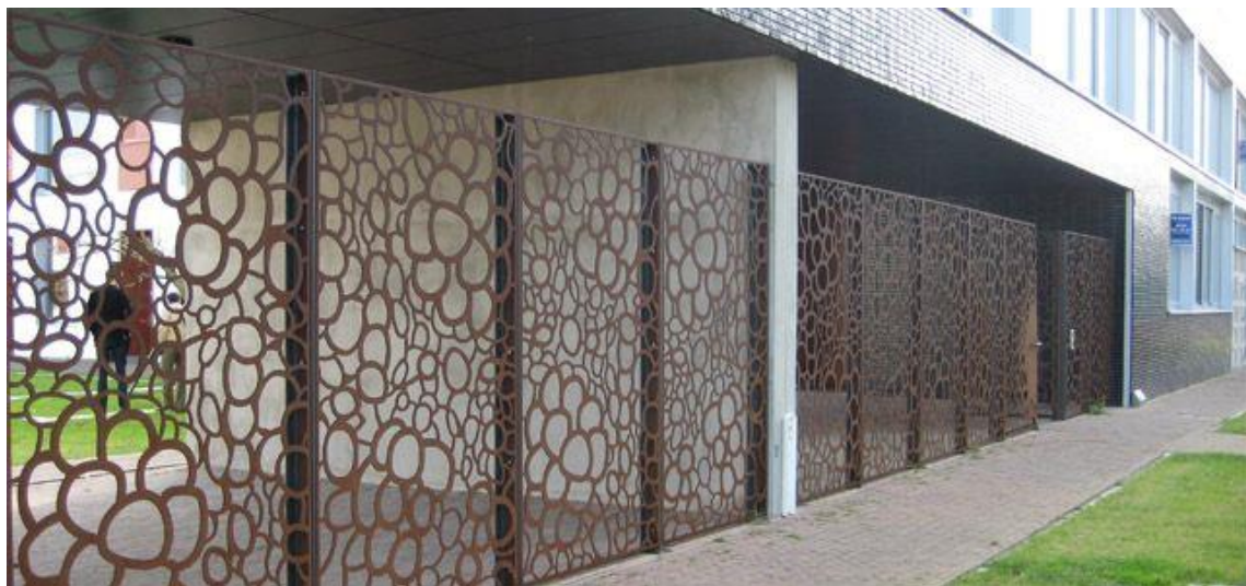
Figure 65 Example of ground level mitigation – porous screens
