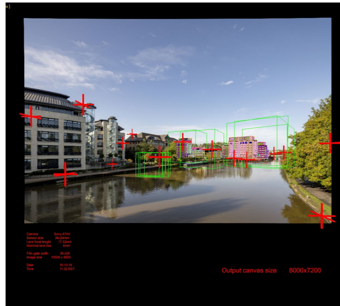
3.7 Screen grab of model matched to photograph
