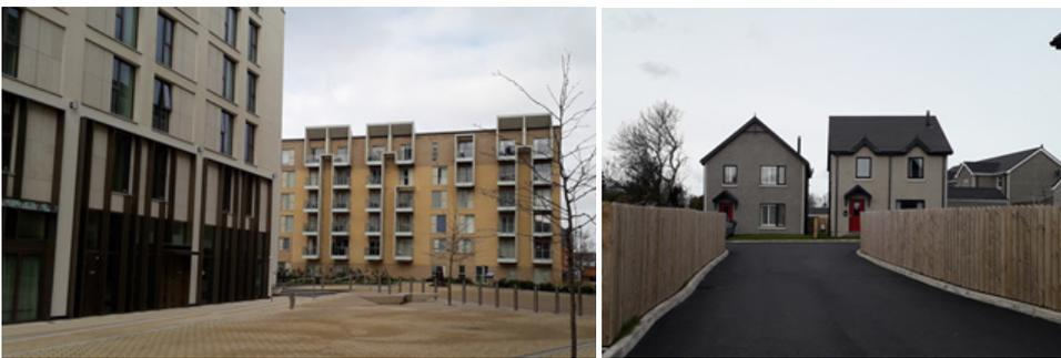
Figure 9-2: Example of light-coloured (high albedo) facades and external hard surfaces (left) and tarmac (right). Ground surface temperatures are likely to be lower in the left-hand example than the right with a consequent impact on local air temperatures in hot weather, for a given similar location
