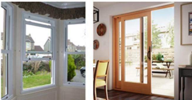
Figure #14-2: Examples of openings providing just under 50% free area: window with bottom half opening; patio door
