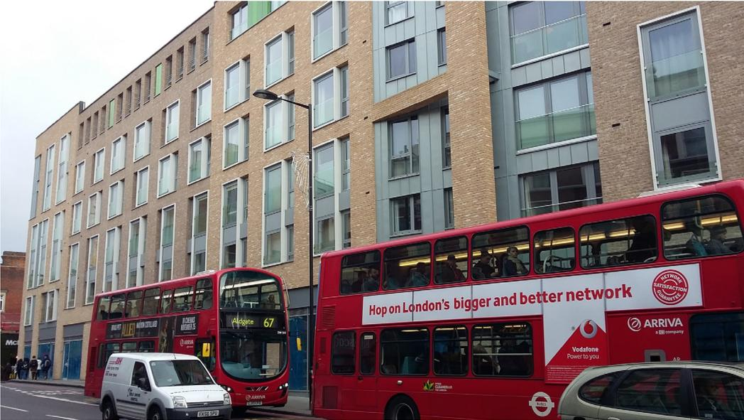
Figure #3-1: The busy road and bus stop in front of this apartment block are likely to make it uncomfortable for occupants to regularly open their windows for long periods of time, due to noise as well as exhaust fume smells.
