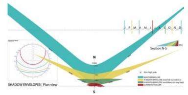
The diagram above shows the shadows of a given height at two extremes, namely end December and end June (winter and summer, blue and red respectively) and two intermediate scenarios (autumn and spring). The green shadow envelope captures shadows cast in the warmer six months of the year approximately between April and September. The yellow envelope demonstrates the impact of overshadowing across a longer annual time span, i.e. a nine-month period between mid-February and mid-November.
