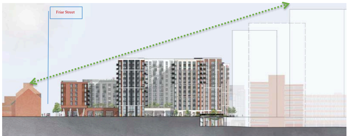
Figure 19 Extract from Station Hill Application DAS Page 100 showing heights stepping up from Friar Street in the south towards the station (Red arrow added for emphasis).
