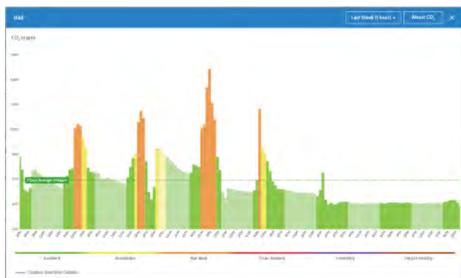
Figure 13 Example of the class indoor CO 2 data, highlighting the increase in CO 2 through the day. Data was collected using a datasheet such as that shown in Figure 3.
