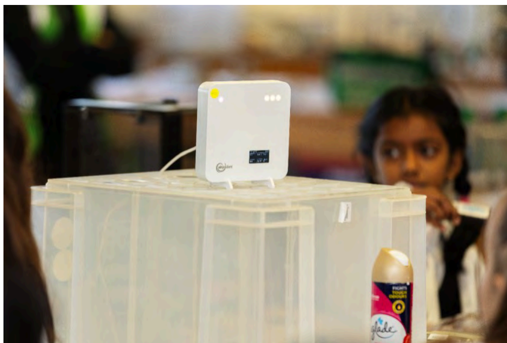
Figure 26: Box used to trap vapour from air freshener to undertake measurements using an AirGradient indoor sensor.
