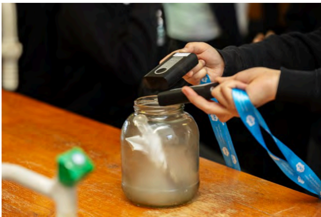
Figure 24: Pupils undertaking particulate matter measurements using Atmotubes caused by smoke created in a jar.
